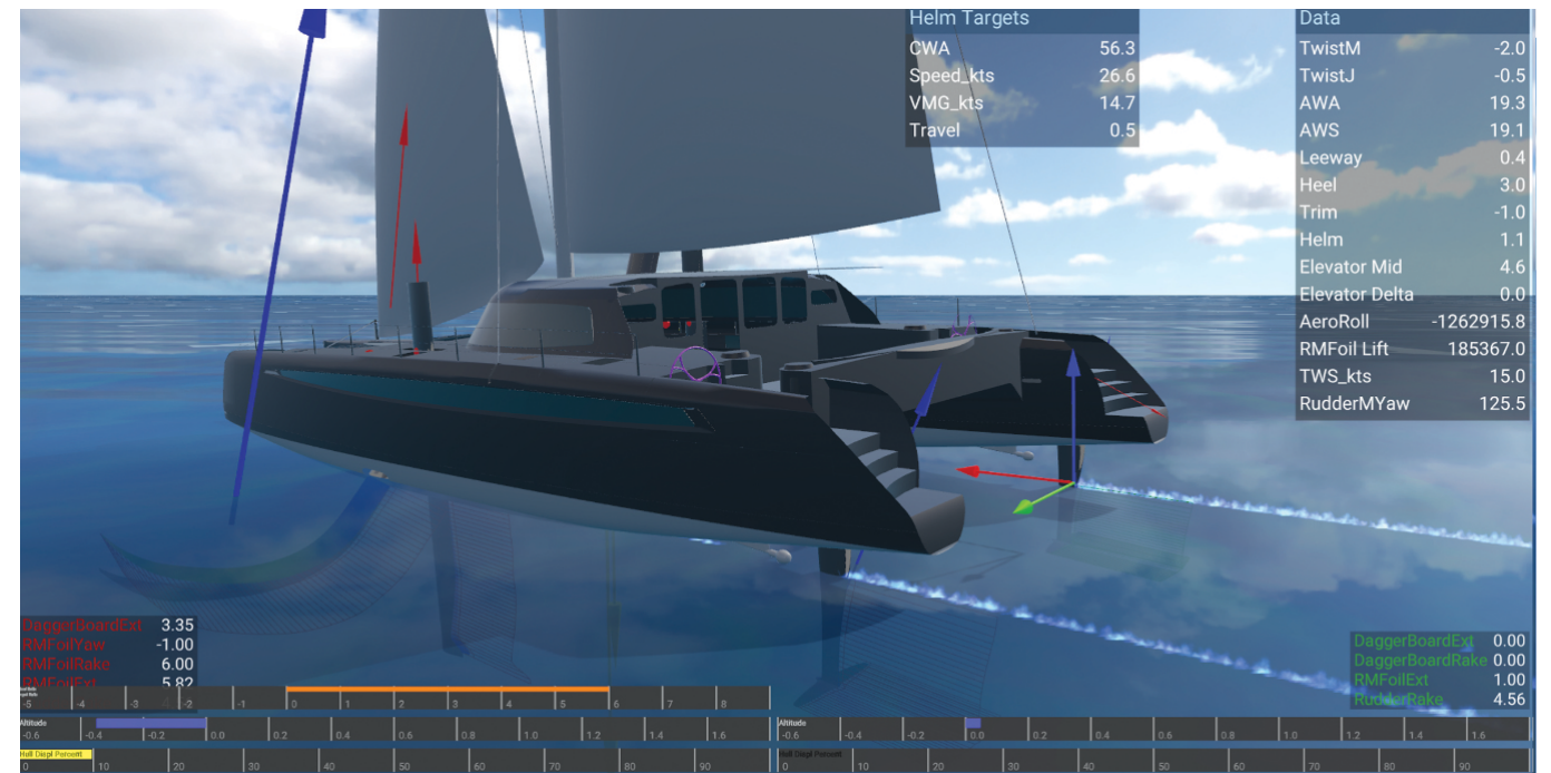
M&M's Gomboc simulator model provides dynamic behaviour predictions and stability insights that inform data-driven design decisions throughout the development process
